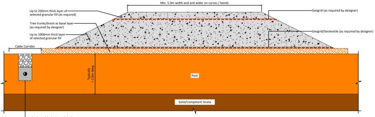
Indicative cable duct trench (only located on one side of roadway across majority of the site). Cable trench can be located on either side of the road surface but where possible it should be located on the upstream side of the road surface.
