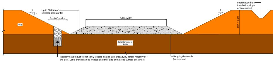
Indicative cable duct trench (only located on one side of roadway across majority of the site). Cable trench can be located on either side of the road surface but where possible it should be located on the upstream side of the road surface.
